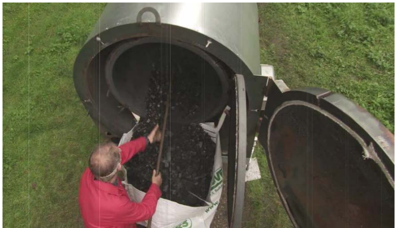
Figure 1. Emptying a load of natural charcoal and biochar from the U.K. licensed, U.S. built, trailer-mounted Exeter retort.
