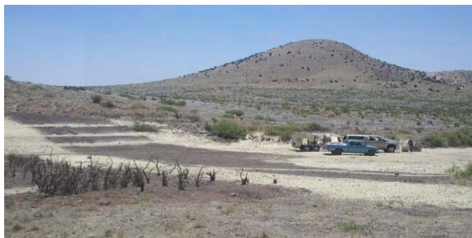
Figure 5. A Zerosion test plot with the product blown onto a mine tailing slope in both broadcast areas and stepped berms. Note the modest size of the application unit: a pick-up towable trailer-mounted blower, water/slurry mix tank, hoses, and pump. The chips were brought in a separate trailer, not shown.
