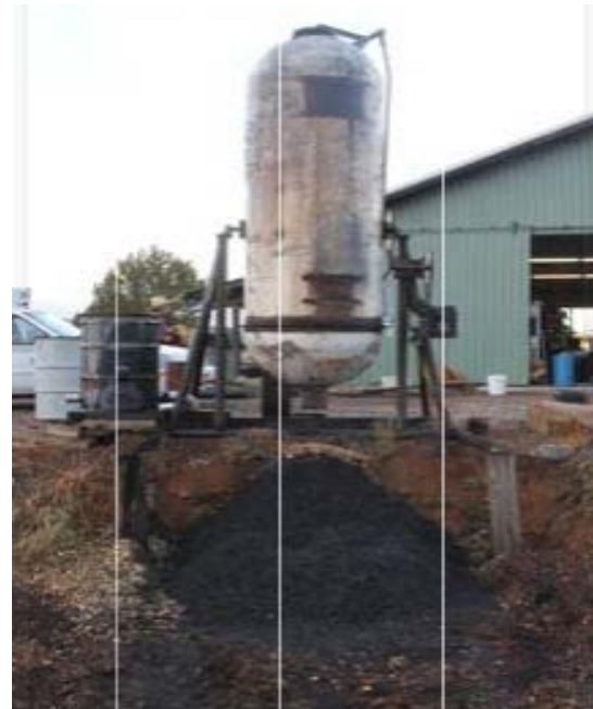
Figure 2. Stationary TLUD-style pyrolysis retort with heat and syngas recovery; made from a 500 gallon propane tank by Restoration Technologies.
